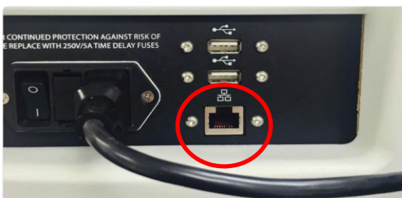
Figure 2: Ethernet (RJ-45) jack location outlined in red.
