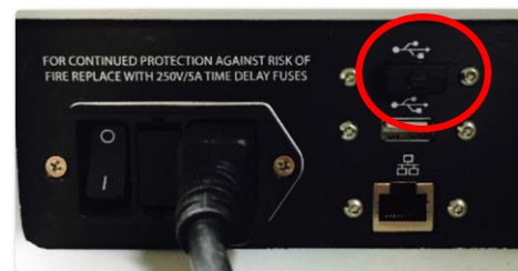
Figure 5: USB Wi-Fi Adapter inserted into an available USB port on the back of the XFP.
