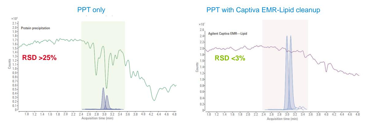
Lipids cause reproducibility problems resulting in high RSD values. Using Captiva EMR-Lipid enables low RSD values and higher peak areas. Higher peak areas due to less ion suppression can lead to lower detection limits.
