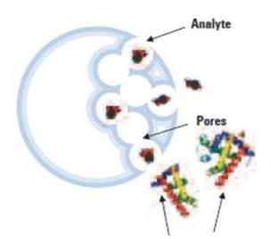
Large endogenous proteins do not bind to the surface of the polymer and cannot access pore structure.
