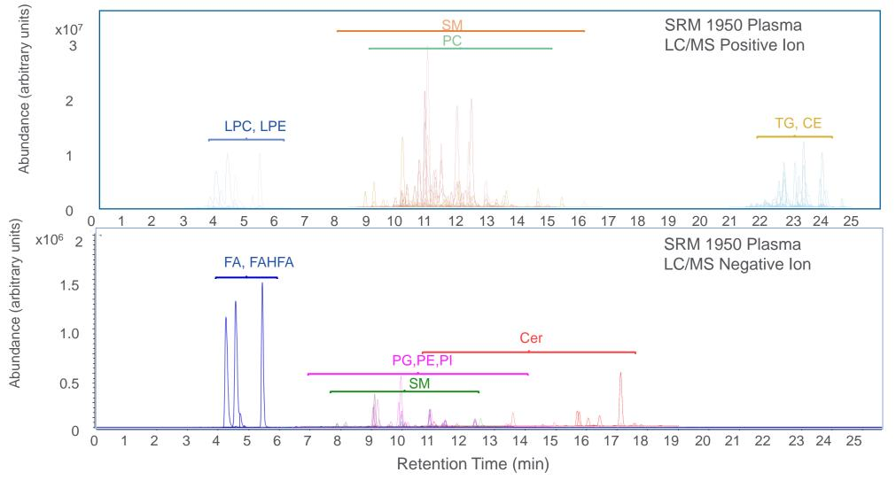
Positive (top) and negative (bottom) extracted ion chromatograms (EICs) for identified lipid compounds in human plasma, using the Bond Elut Lipid Extraction SPE method. (5994-1783EN)
