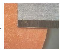
Stuck septa particles can cause sealing problems on next septum installation. Talc can cause activity/trap plugging problems
