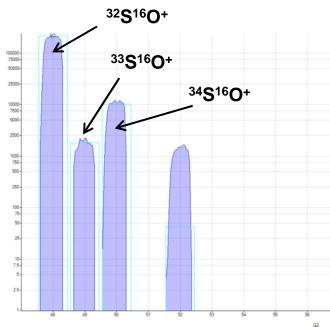
Single-quad can also do SO mass-shift to move S (as SO $^+$ ) away from the  $O_2^+$  interference.
