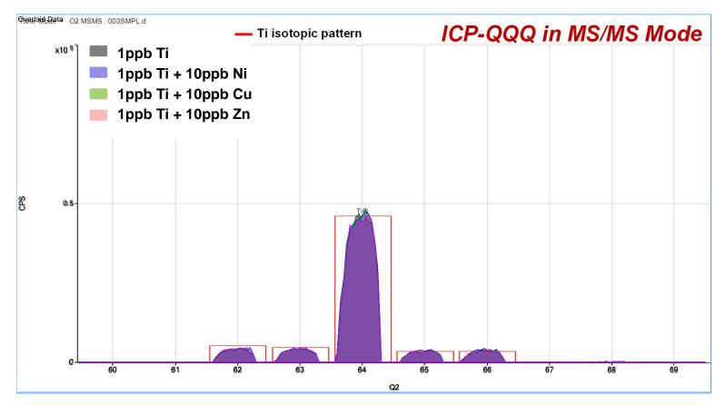
MS/MS mode allows Ti to be measured as TiO with no overlap from Ni, Cu, Zn
