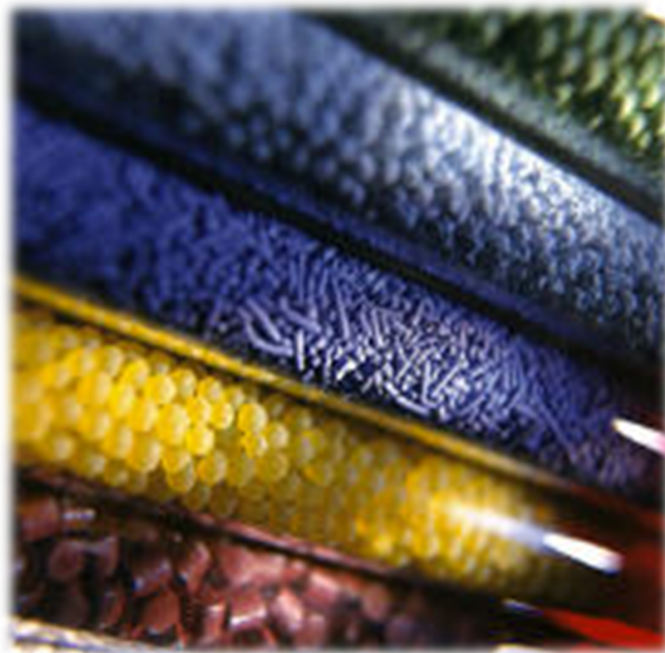
Catalysts used in catalytic cracking or reforming
