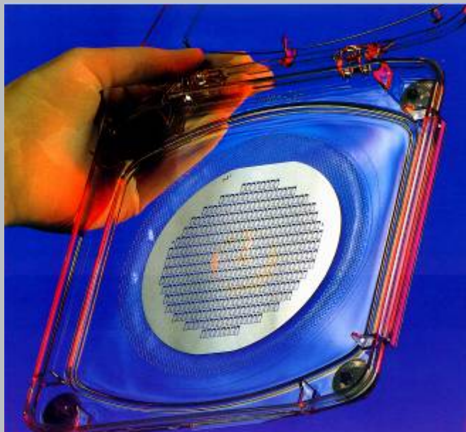
4-inch wafer with 388 probes
