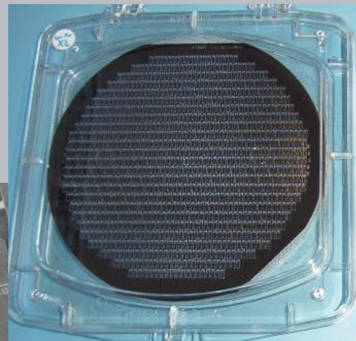
6-inch wafer with more than 1000 probes
