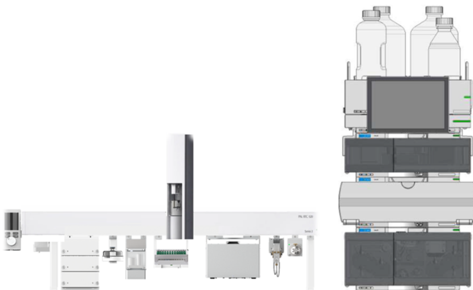
Figure 1: The image illustrates the required space next to the PAL3. Make sure there is sufficient space for unobstructed Y-axis movement of the PAL3. For an Infinity III System, a footprint Depth 436 mm (~17,2 inch)/ Width 396 mm (~15.6 inch) is required shown above. (Note: Not drawn to relative scale)
