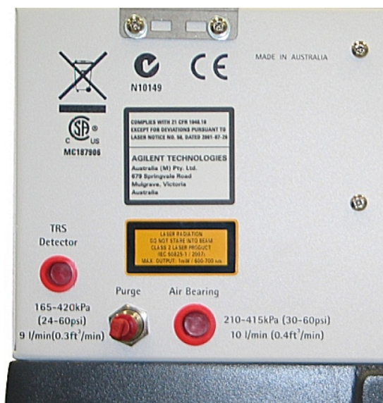
Figure 1. Laser safety label locations on the rear of the Agilent Cary 600 Series FTIR spectrometer
