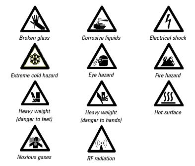
The following symbol may be used on warning labels attached to the instrument. When you see this symbol, refer to the relevant operation or service manual for the correct procedure referred to by that warning label.
