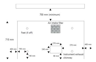
Figure 3. Top view of instrument
