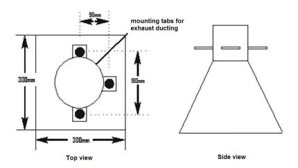
Figure 8. Exhaust ducting details
