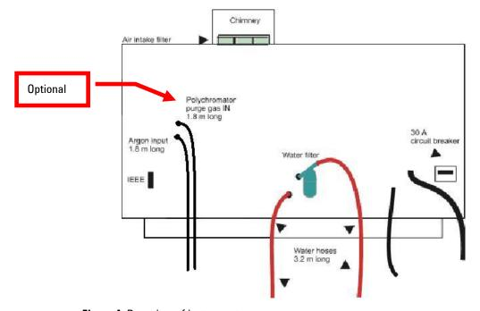
Figure 4. Rear view of instrument
