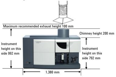
Figure 6. Spectrometer and flue position
