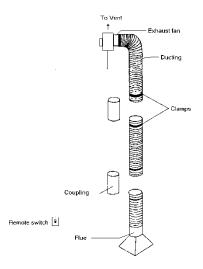
Figure 7. Agilent exhaust kit components
