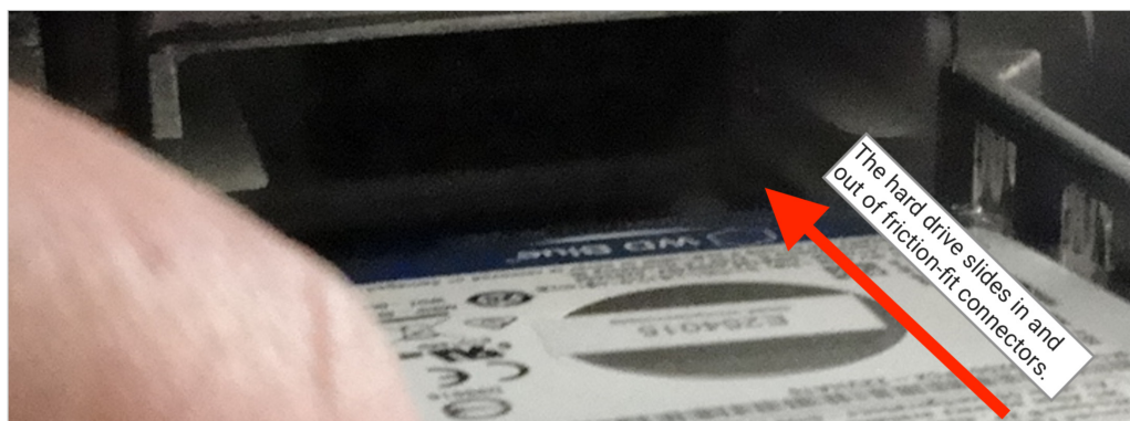
Figure 15. Installing the new solid-state drive into the same bottom position.
