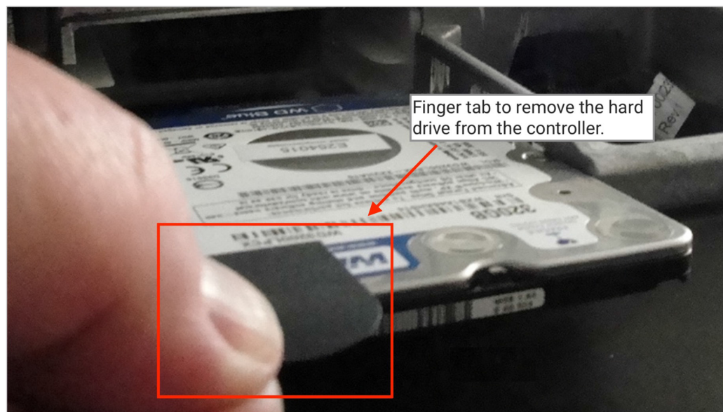
Figure 14. Gently pulling the hard drive finger tab.
