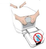
**CAUTION**: Do not use the front end of the Loader as a lift point. Using the Loader to lift the device can damage the baseplate, which is easily bent.
