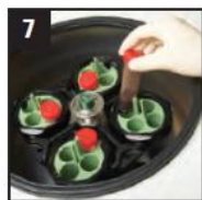
7 Centrifuge at 4000 rpm for 5 minutes
