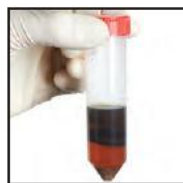
Phase separation of acetonitrile and aqueous layer
