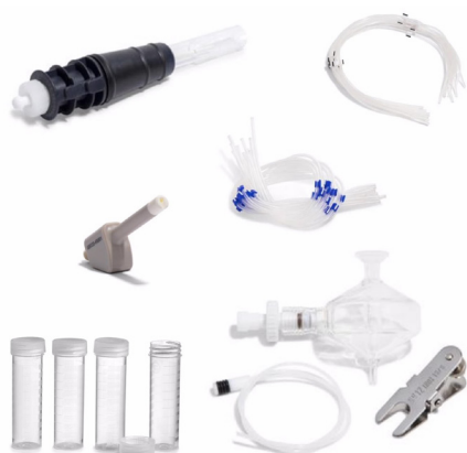
Figure 6. Lithium-ion battery sample introduction kits suitable for Agilent 5800 series ICP-OES instruments. The kit includes the recommended torch, spray chamber, nebulizer, peri-pump tubing, and sample tubes.
