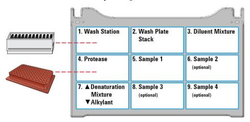
At deck location **7**, ensure the **Denaturation Mixture** plate is stacked atop the **Alkylant** plate.
