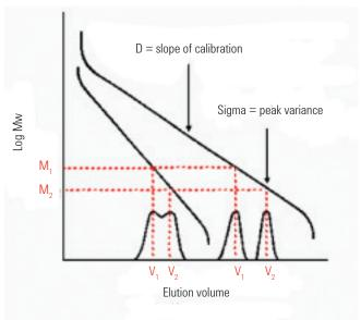
Figure 3. Calculating the resolution factor.
