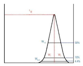
Figure 4. Calculating peak symmetry.
