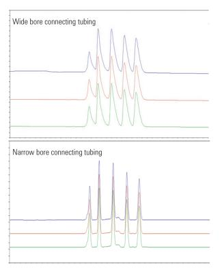
Figure 5. Narrow bore tubing improves peak shape in GPC/SEC, compared to wide bore tubing.
