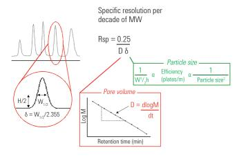
Figure 2. Calculating specific resolution per MW decade across all MW regions.
