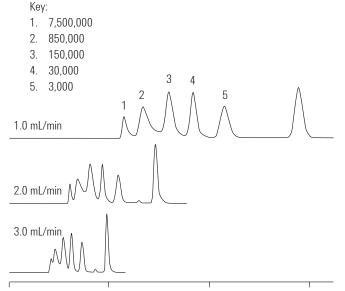
Figure 6. Take care to choose the best flow rate, depending on the particle size of the column
