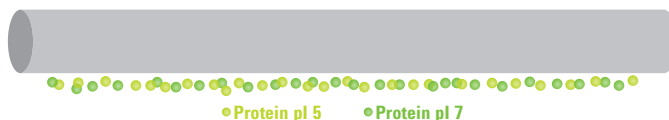
Figure 2.1 A mixture of carrier ampholytes and sample proteins is filled into the separation capillary. The grey color indicates premixing.
