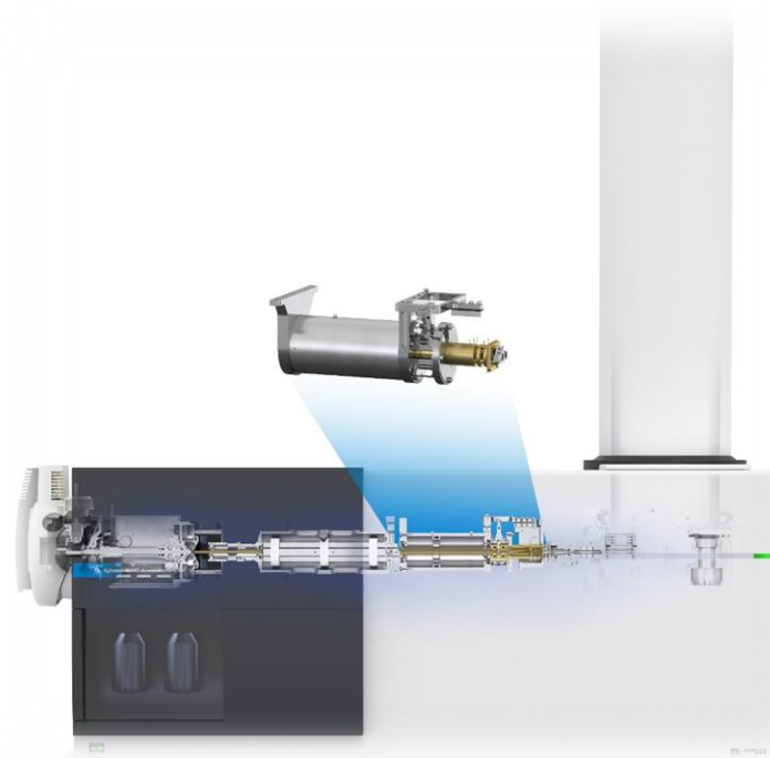
Figure 2. An instrument schematic showing the Agilent 6545XT AdvanceBio LC/Q-TOF equipped with an ExD cell for electron fragmentation.
