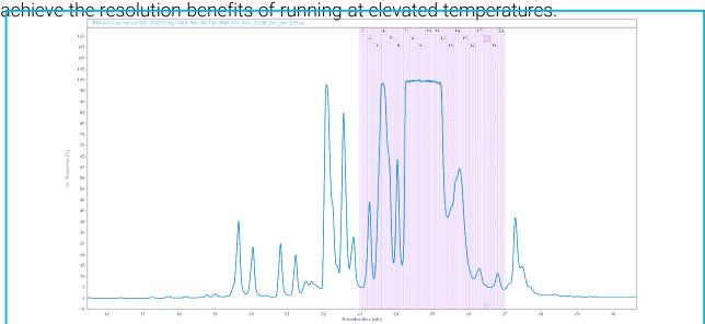
The figure above shows an optimized semi-prep separation of a crude oligo sample run at  $60^{\circ}\text{C}$  on an AdvanceBio Oligo 10x150mm column. Utilizing the gradient to focus the sample at the head of the column, a quad injection, of  $160~\mu\text{L}$  (3.2 mg) total is loaded onto the column. The fractions were collected and analyzed on an analytical column to demonstrate purity and yield in the figure below.
