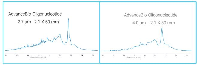
As demonstrated in the figure above, the AdvanceBio Oligonucleotide column chemistry is easily scalable across the 2.7 and 4  $\mu$ m particle sizes for a crude sgRNA sample allowing for easy method transfer and scale up.
