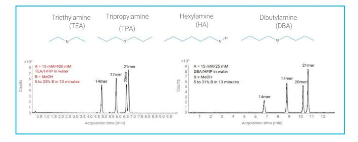
Significant improvement of resolution and sensitivity can be obtained by careful development and optimization of your method. Depending on the ion pairing reagent that you choose and the concentration, it will influence the retention and separation on column. More hydrophobic ion-pairing agents will increase retention and can be used to separate the target product from close eluting impurities.
