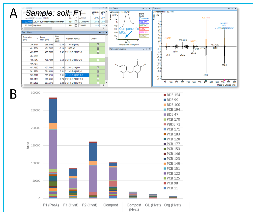
Figure 5. PCBs and PBDEs in soil DCM extracts. (A) An example of BDE detected in soil from Field 1 at the time of harvesting. ExactMass table (bottom left panel) shows how well the accurate mass fragment ions are matching the unit mass library hit providing the additional confirmation of compound ID. The most representative ions are highlighted in mirror plot when m/z matches the library hit formula. (B) Bar graph showing responses of PCB and PBDE for all the soil samples they have been identified.
