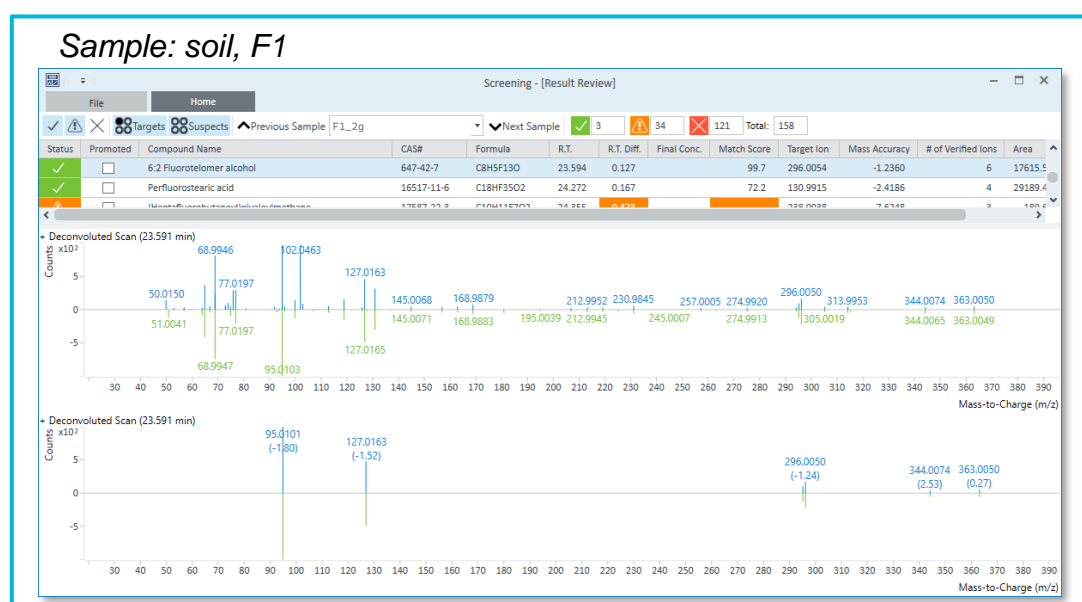
Figure 3. 6:2 FTOH detected in soil using SPME and PFAS PCDL-based screening approach. The mirror plot at the top shows deconvoluted compound spectrum versus the spectrum from the PFAS PCDL. The mirror plot at bottom displays only target and qualifier ions with mass accuracy in the parentheses.
