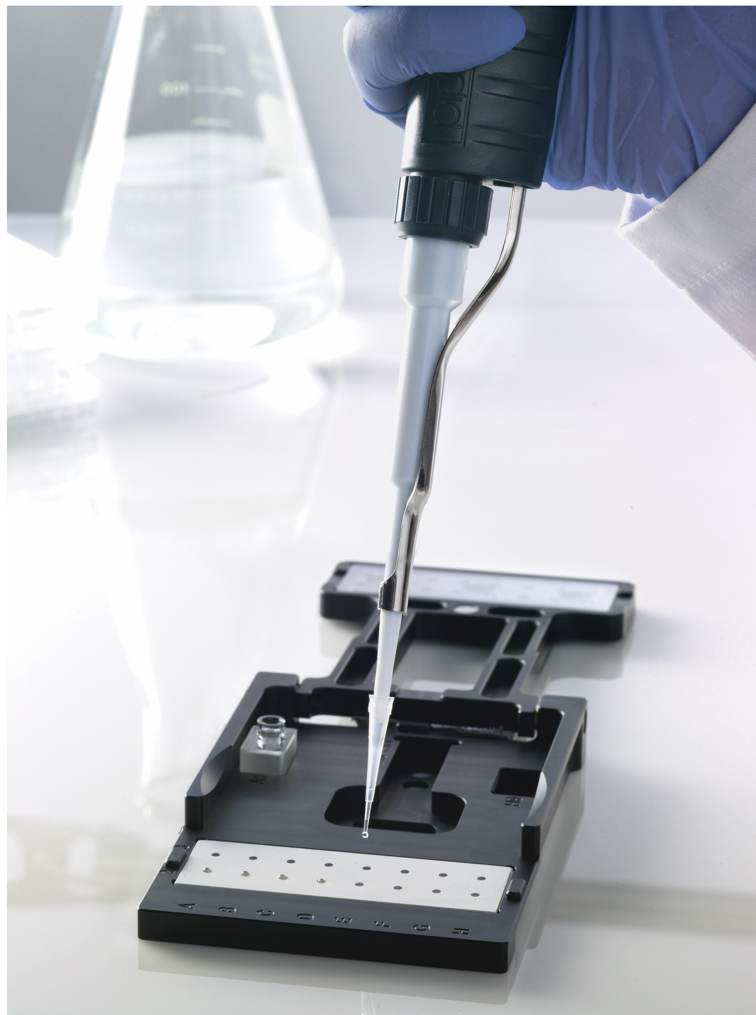
Figure 2. The Agilent BioTek Take3 microvolume plate with 16 microspots (2 µL) for microvolume measurements. The plate can also accommodate two BioCells, and a standard 1-cm pathlength cuvette.
