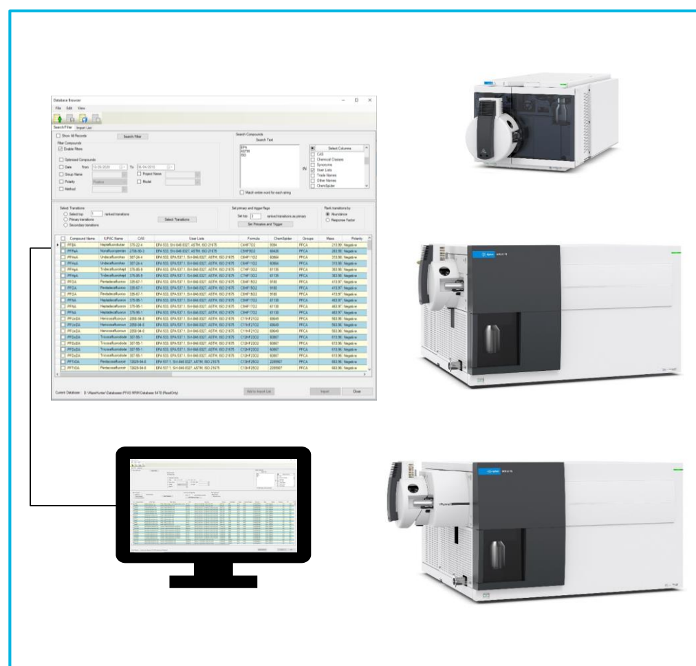
Figure 1. Databases are fully integrated with the MassHunter LC/MS Data Acquisition software to facilitate quick development of data acquisition method and expansion of the analyte list.
