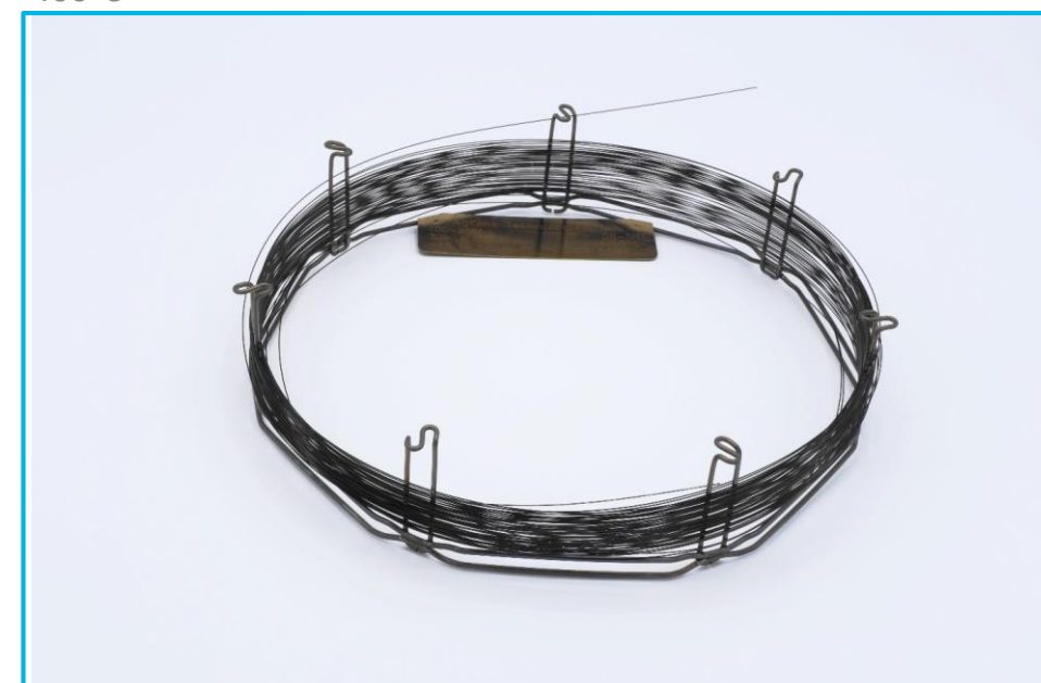
Figure 4b. Agilent J&W DB-5ht GC Column after 25 hours operating at 400°C
