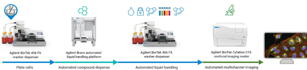
Figure 1. Conventional Cell Painting assay workflow from cell seeding to image collection, and the proposed Agilent automation solutions supporting the various steps of the process.
