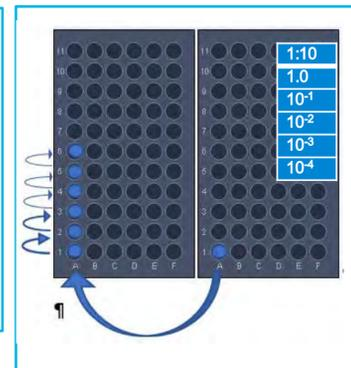
Figure 3: Injector Program Schematic
