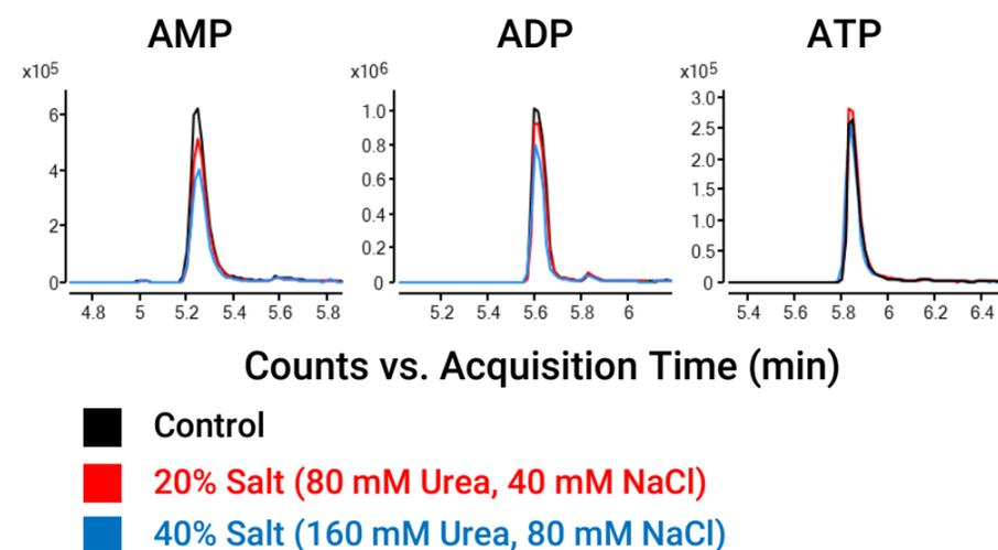
Figure 3. Metabolite standards were spiked with salt that was equivalent to 20% and 40% of salt concentrations found in human urine. Higher salt concentrations (>40%) were not attempted because the salt was not soluble in the sample matrix (80% ACN).
