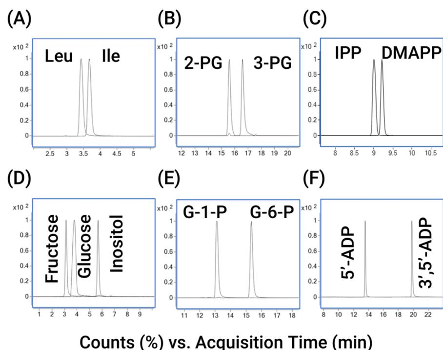
**Figure 2.** Chromatograms of structural isomers separated by HILIC LC/MS method.
