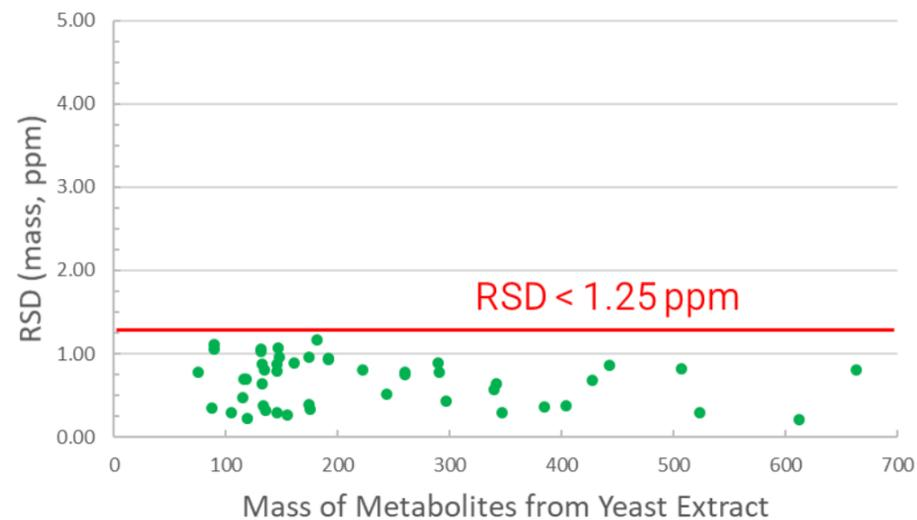
**Figure 6.** Excellent mass accuracy stability over 18-hour assay time for metabolites extracted from yeast. The (A) average absolute mass error was  $\leq 1.5$  ppm and (B) RSD of mass error was  $\leq 1.25$  ppm ( $n = 47$  metabolites) in negative ion mode.
