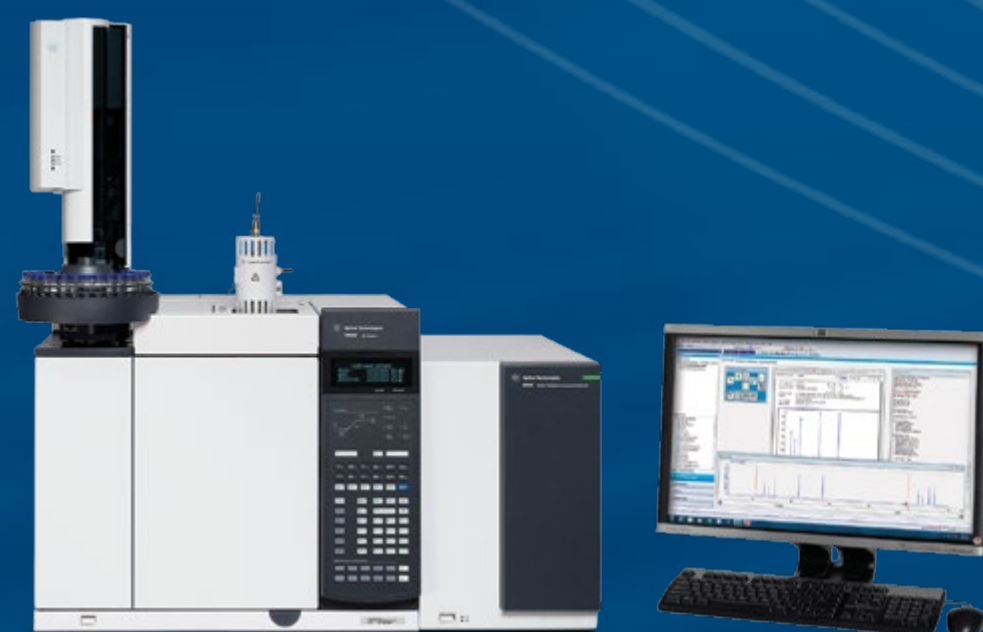
Fully integrated Agilent 8355 SCD with Agilent 7890B GC and OpenLAB Chromatography Data System software High selectivity and sensitivity for complex trace-sulfur methods
