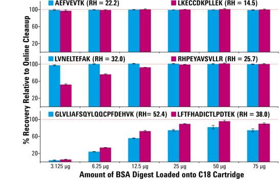
BSA digests were loaded onto C18 cartridges (n = 3) at different concentrations to generate the indicated load mass. Signals normalized to online cleanup of 1.25  $\mu$ g of the same digest at highest tested concentration (0.75  $\mu$ g/ $\mu$ L).
