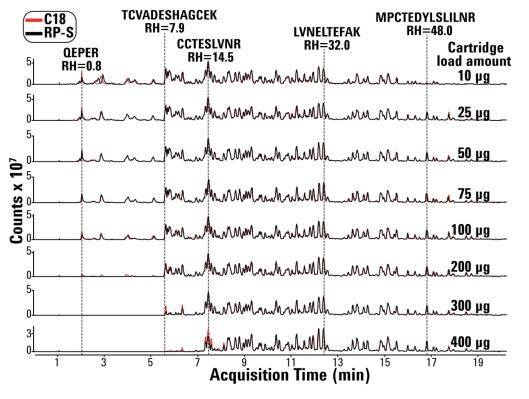
Various amounts of tryptic BSA digests were cleaned up with C18 and RPS cartridges. The TIC from these experiments show:
