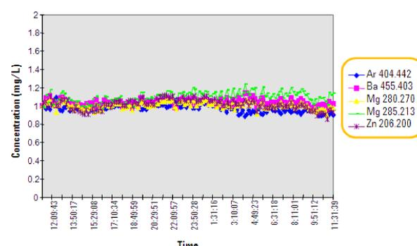
**Fig 3.** Stability in 20% NaCl using the Agilent sheath gas torch
