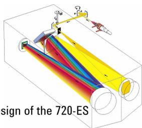
**Fig 1.** Optical design of the 720-ES
