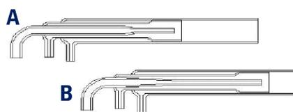
HDS torch (B) provides more laminar pathway for the aerosol reducing salt build-up in injector at a specific point.
