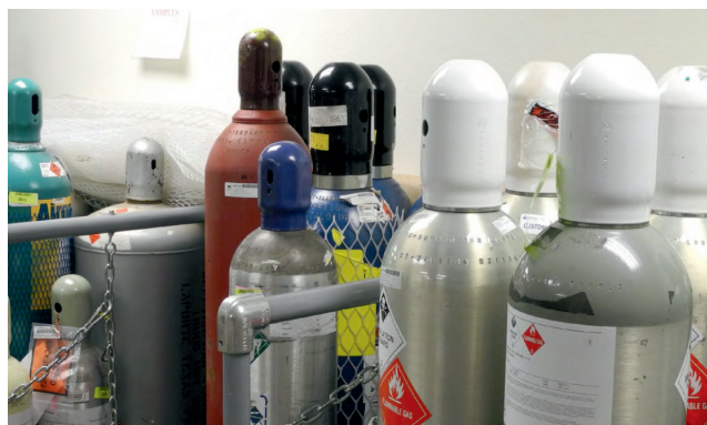
Figure 1. Many semiconductor gases are toxic, flammable, or pyrophoric, so require specialized GC sample introduction.
