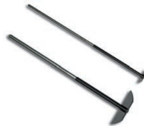
Standard paddle (top) with compendial paddle (bottom) with noncompendial mini paddle
