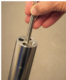
Figure 2: USP Apparatus 6 (rotating cylinder)
