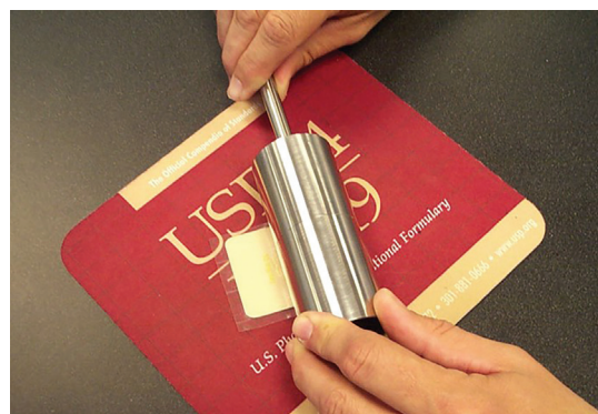
Figure 5: Mounting TDS onto rotating cylinder
