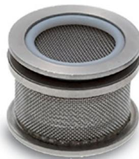
Sinker basket, with cover, 40-mesh, 381 µm
