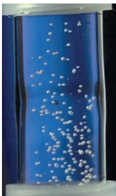
Figure 1. Theophylline Beads floating freely within the Reciprocating Cylinder exposing all surfaces to the media.
