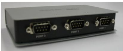
**Figure 4.** Four-port, USB-to-Serial converter
