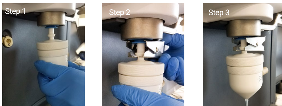
Figure 4. Installing the inert spray chamber onto the MP-AES inert torch.
