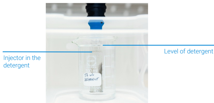
Figure 2. Ensure that the injector and outer tube are immersed and soaking in the detergent solution
