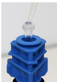
Figure 4. Pipette some of the acid solution through the open-end of the ball joint to flush the injector
