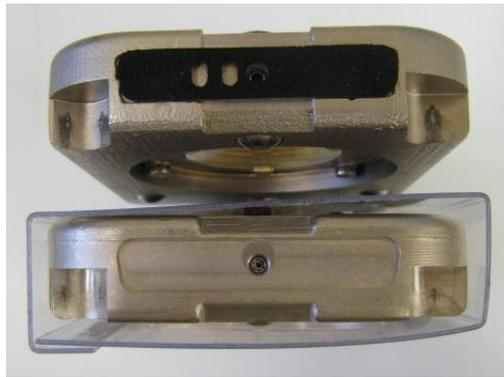
**Fig 1** – Underside of the beamsplitter shown with and without the ID label
