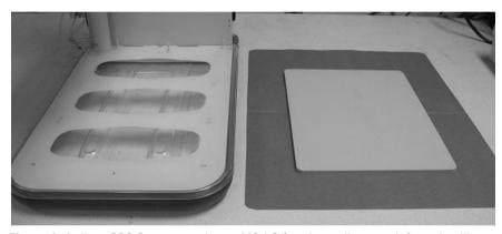
**Figure 1.** Agilent SPS 3 autosampler or 440-LC fraction collector—left; and spill tray support plate—right
