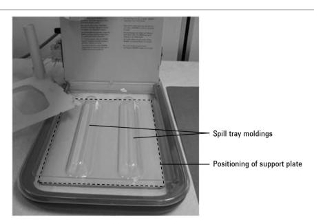
Figure 2. Correct alignment of the support plate
