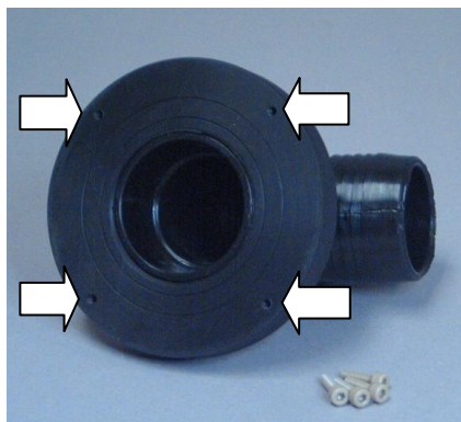
Figure 2. Exhaust piece holes to align with holes on the Agilent SPS 3 cover
