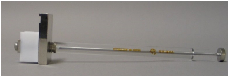
Figure 4. The syringe and T-piece assembly
