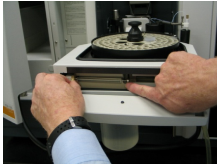
Figure 6. Replacing the syringe block assembly and syringe
