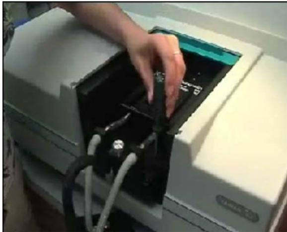
**Figure 4.** Tightening the front holding screw
