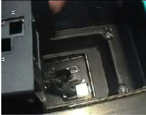
**Figure 3.** Connecting the two plugs on the accessory to the two sockets located in the base of the instrument. Note that the 6 x 6 Multicell Holder is pictured, however the installation procedure is the same for the 8 x 6 Multicell Holder.
