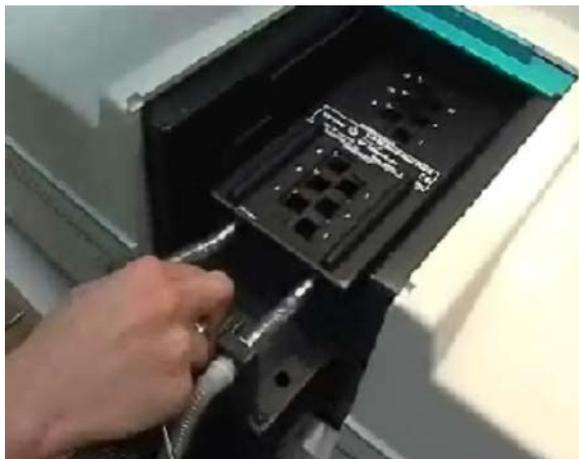
**Figure 5.** Sliding the top half of the accessory forward. Note that the 6 x 6 Multicell Holder is pictured, however the installation procedure is the same for the 8 x 6 Multicell Holder.
