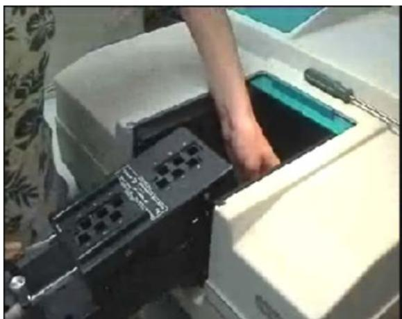
**Figure 2.** Resting the Multicell Holder accessory on the edge of the instrument. Note that the 6 x 6 Multicell Holder is pictured, however the installation procedure is the same for the 8 x 6 Multicell Holder.
