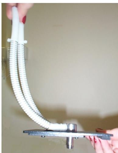
**Figure 1b)** The baseplate with tubing that sits in the Extended Sample Compartment. You will also receive hosing to connect to the water bath hoses.
