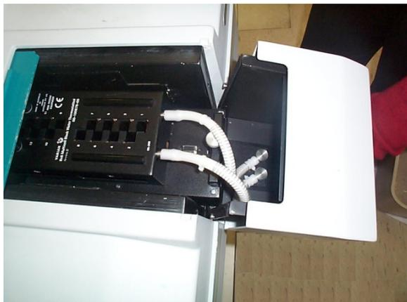
**Figure 7.** Attaching the Extended Sample Compartment to the instrument
