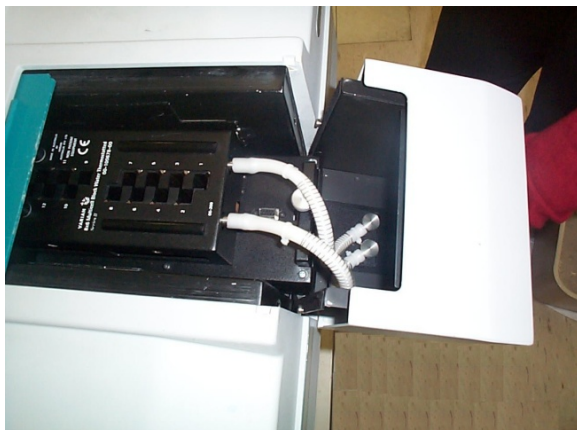
Figure 6. Attaching the Extended Sample Compartment to the instrument
