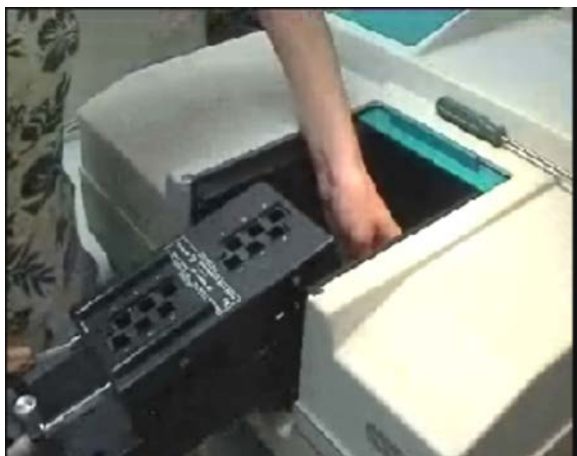
Figure 1. Resting the Multicell Holder accessory on the edge of the instrument
