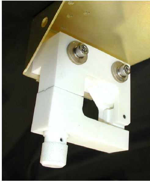
Figure 5. Torch clamp assembly secured to mounting bracket using standoffs with M6 screws, spring washers and flat washers. For clarity, this picture shows the bracket outside of the instrument. You DO NOT need to remove the bracket from the instrument.
