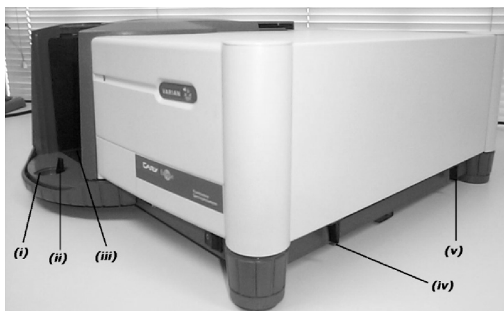
Figure 4. (i) Circular cover plate (removed) (ii) Front black clasp (iii) Sample compartment front door removed (iv) Right hand side black plastic clasps. Here three of the five black plastic clasps have been flipped up in order to release the cover. The remaining two clasps are located in the same position as (iv) and (v) on the opposite side of the instrument.
