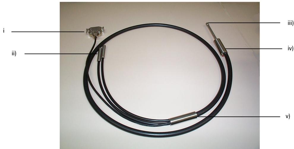
**Figure 2.** Fiber Optic Probe. i) Cable plug. ii) Connector ends. iii) Probe tip. iv) Remote read button. v) Metal join.
