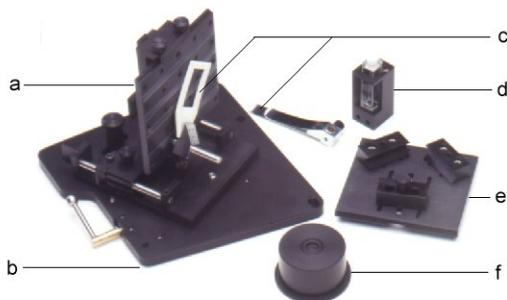
**Figure 1.** The Solid Sample Holder accessory.
