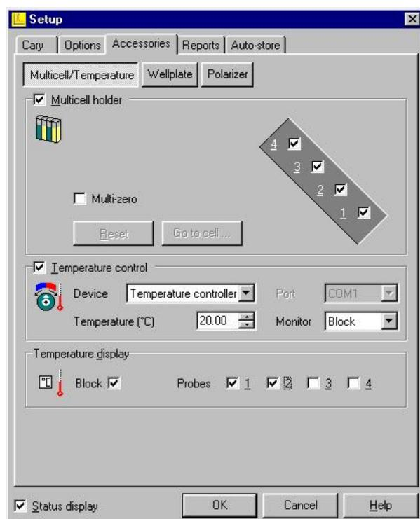
**Figure 2.** Accessories tab showing a typical setup of the multicell holder accessory
