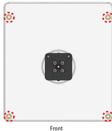
Figure Mounting holes on Labware MiniHub base (top view)
