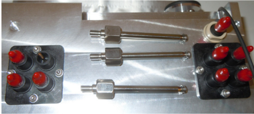
Figure 2 Ion Funnel Optics Assembly and Ion Funnel Drive Module
