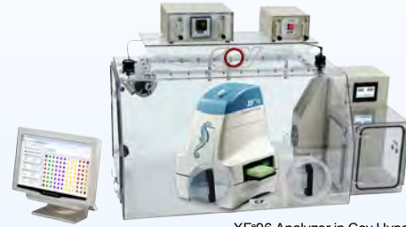
XF96 Analyzer in Coy Hypoxic Chamber. (XF Controller operates outside.)
